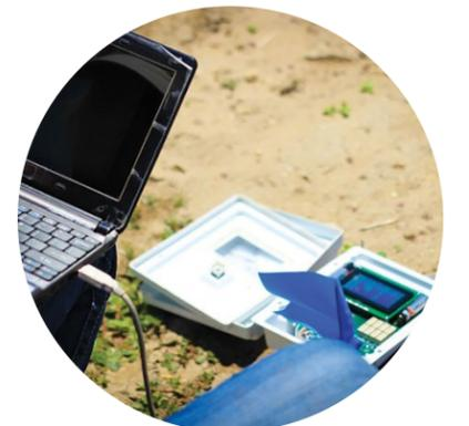
Pictured is the computer connected to the soil sensors to collect and store moisture readings directly from the field. The information will be used to make an informed irrigation decision.
